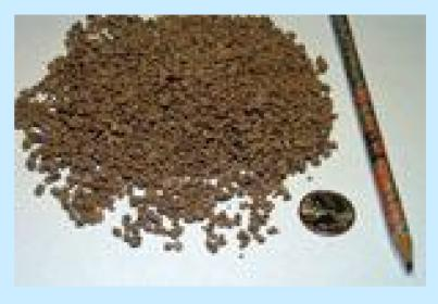
The EversTech Process plant in Fresno, CA, owned by Cottonwood Creek Biosystems, takes in tankered grease and food processing wastes and generates single cell protein and dischargeable water. Sample of the single cell protein biosolids after the drum dryer. Sample of the single cell protein biosolids after the drum dryer.
